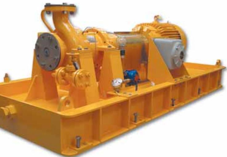
In densitometer applications, the sampling pumps have to be able to take the full pressure from the main pipeline (up to 2 metres / 80 inches diameter) sample the liquid and then return it to the pipeline. System pressures of up to 185 bar have to be contained, the cost of a mechanical seal that would have been able to handle these pressures would be considerable.
